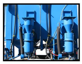
Aboytes Mfg. Cyclone Vortex Reclaiming Systems are designed to keep abrasive media free of contaminants while minimizing media waste.
